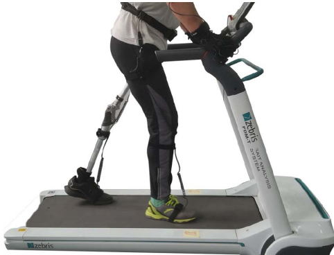
Fig. 4. Hip disarticulated amputee test on the treadmill.
